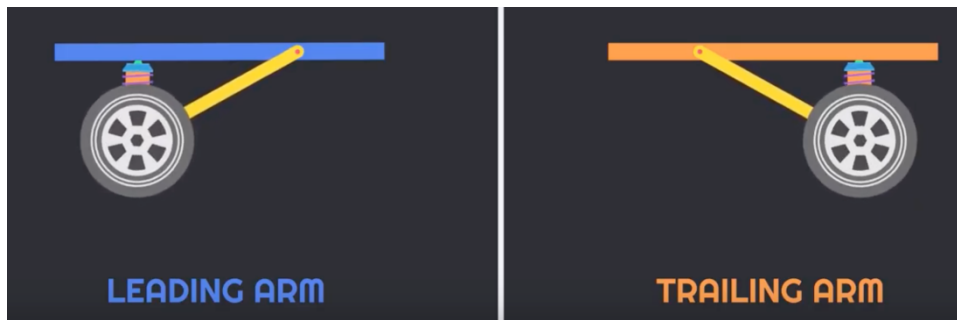
Figure 7: Trailing Arm vs. Leading Arm Diagram
