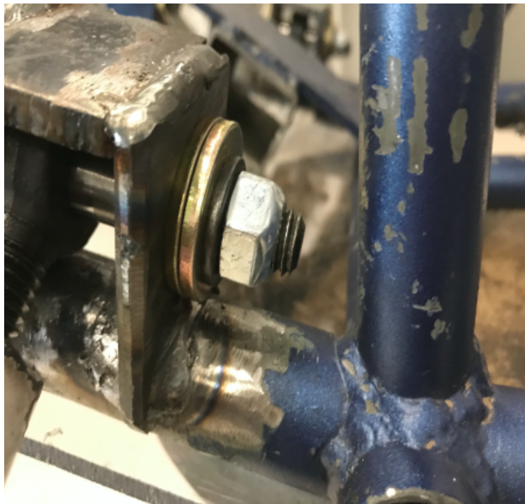
Figure 43: Steel welded on the front suspension
