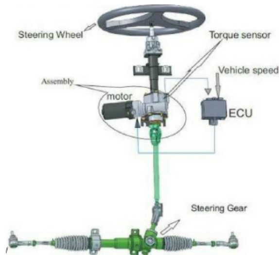
Figure 14: Electric Power Steering Setup [30]
